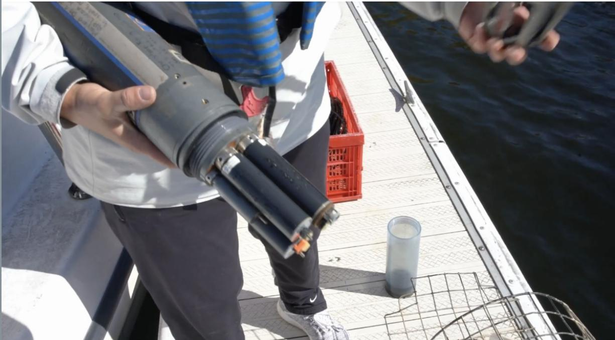
The water quality meters do many essential tasks at the same time. They measure the water flow and content from the watershed and all aspects of the water in the lake on a continuing basis; they use remote recordings for each area of the lake to set baseline readings for those areas, then detect and compare changes over time; they recognize the
